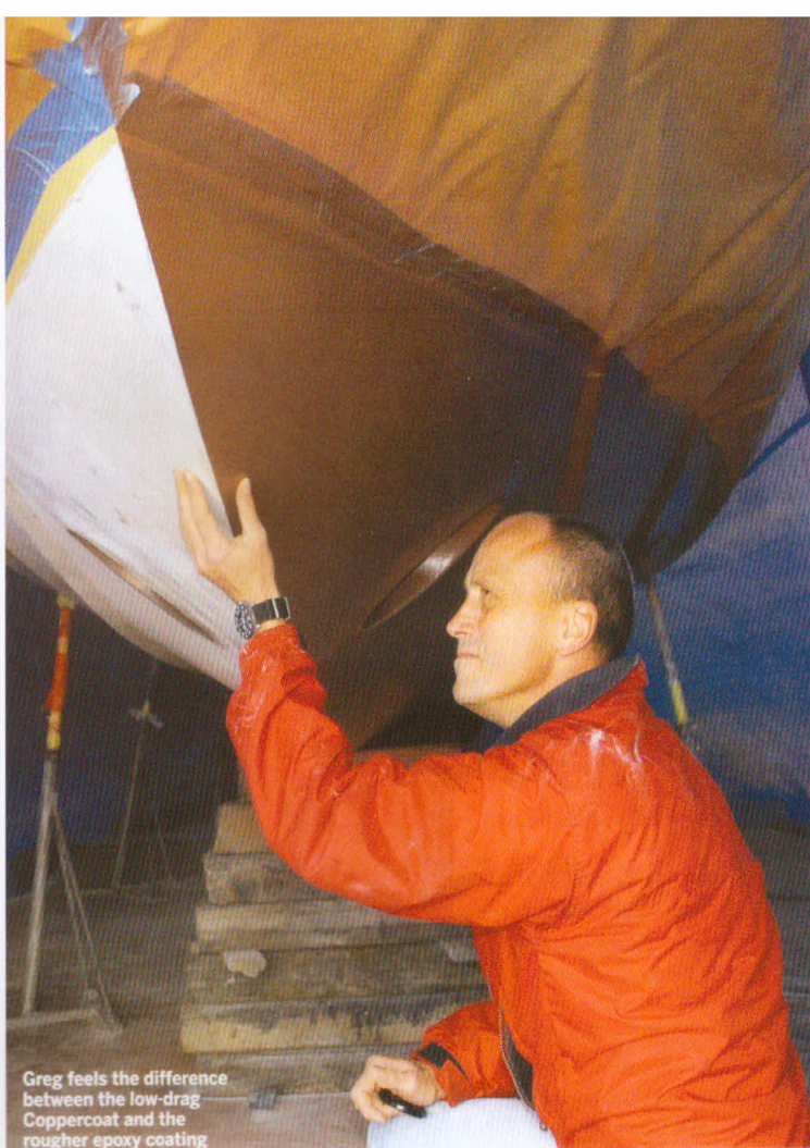
It took two men 30 minutes to lightly abrade the finished surface and expose the copper granules
