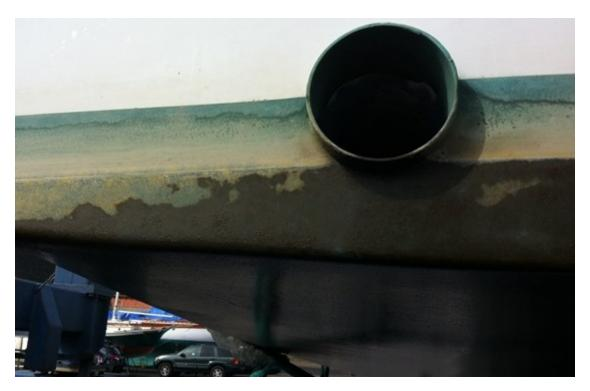
A Coppercoated transom emerges from Long Island Sound -- a high fouling zone. The bottom had been sponged twice underwater during the season, then left alone for the last two months. A light layer of soft slime covered parts of the bottom, but there was no hard growth.
