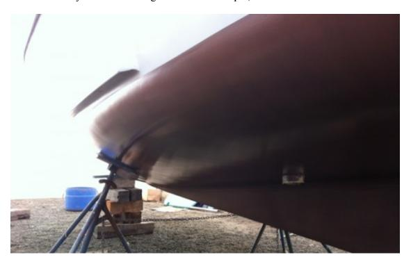
Freshly applied Coppercoat shows a bright metallic color. It's sanded before launch to expose a layer of copper at the surface. Because new copper is exposed by the very slow breakdown of the Coppercoat shell over the years, resanding is not necessary. Underwater sponging and post-season pressure-washing maintain the surface. All photos: Doug Logan
